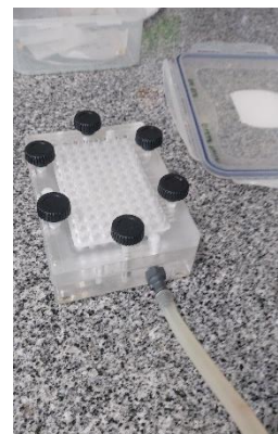
Figure 2. 8: Photo of the completed Dot blot apparatus
